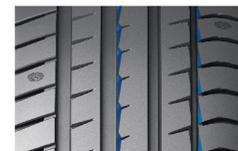
**The transverse pattern groove adopts unique chamfering technology and narrow width design technology**
